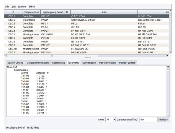
• Coordination tab: Select a lattice site (atom position) and display a chart with the nearest neighbors, next-nearest neighbors, etc. (requires that structure records have atomic coordinates) Define for which constituting Atom: the coordination shell should be calculated, the corresponding Distance cutoff (A): in Å and confirm with Refresh
